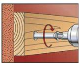
4. The screw is screwed-in until the head of the screw touches the sleeve. The anchor is correctly mounted, when the head of the screw fits tight on the surface and cannot be screwed-in any further.
