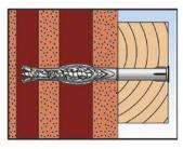
5. Correctly installed anchor in hollow masonry.
