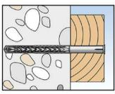
6. Correctly installed anchor in concrete.
