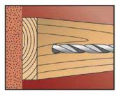
Drill the bore hole acc. to Table B2.1 using the drill method described in the corresponding Annex C.
