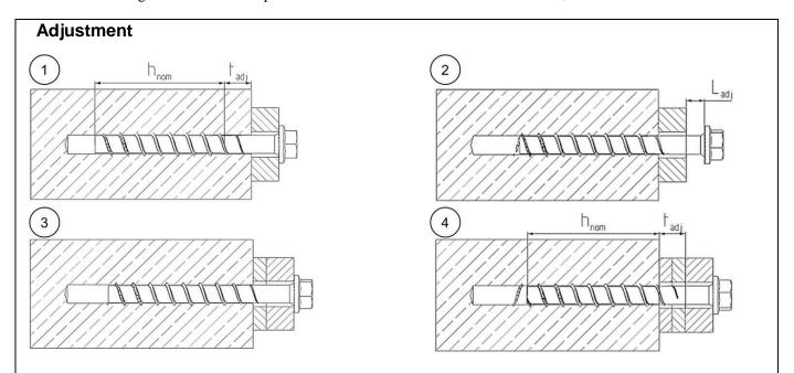
It is permissible to untighten the screw up to two times for adjustment purposes.
