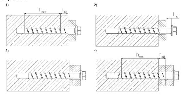
It is permissible to untighten the screw up to two times for adjustment purposes.
